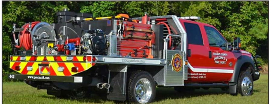
Precinct 4 VFD brush trucks carry a wide array of tools including fire rakes, chainsaws, backpack pumps and drip torches (for controlled burns or back fires). Other tools include a special axe/adz combination called a pulaski and a fire flapper, a rake/broom combination.
